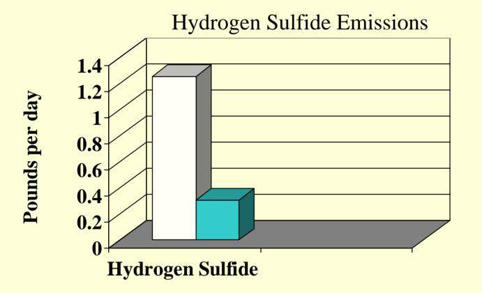
Hydrogen Sulfide Emissions are reduced by 76% as a result of odor control project
