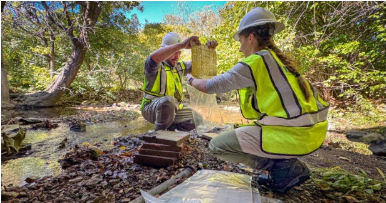
Engineering staff prepare an algae tile pulled from Goose Creek for lab processing
