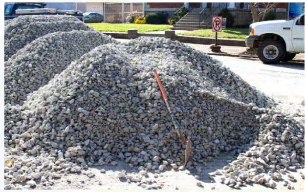
Stone used as base layer for green infrastructure
