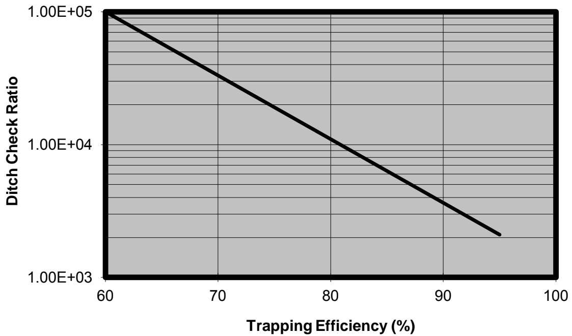
Figure 12.3a. Design Aid for Estimating Trapping Efficiency of Rock Ditch Checks with Fine Texture Soils.
