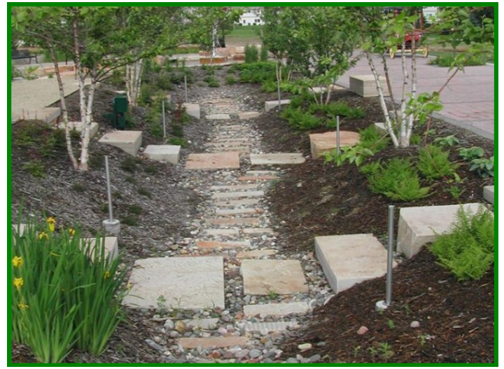
Stepping stones allow accessibility across this linear rain garden/bioswale
