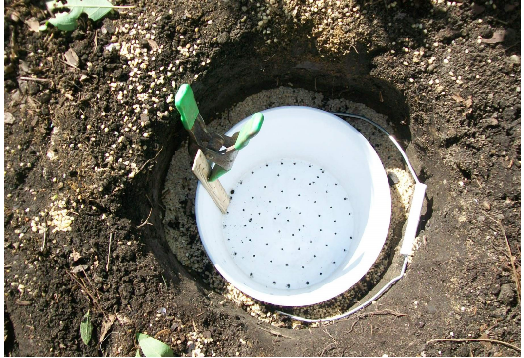
Single-ring infiltrometer infiltration test. (Photo: URS)
