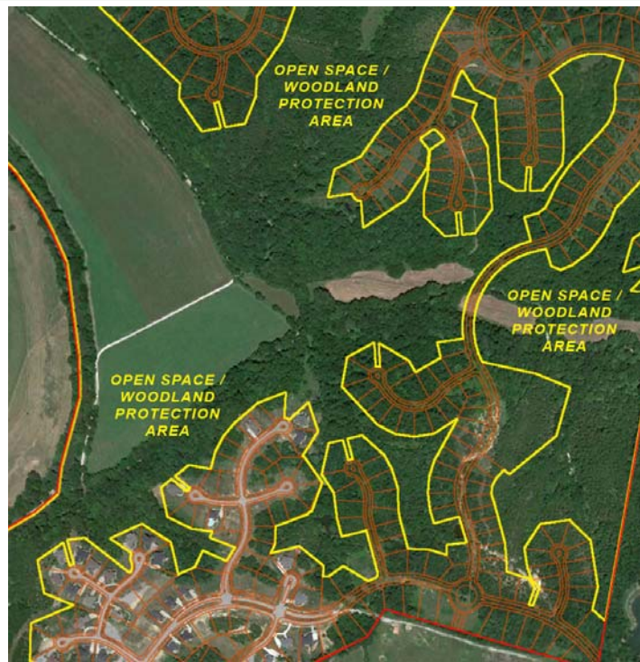
Figure 18.2.4-E. Conservation design is used to preserve open space and natural site characteristics. This approach can reduce the WQv that must be managed on a site.
