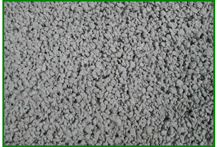
Pervious concrete surface (Photo: Kentucky Concrete Pavement Association)
