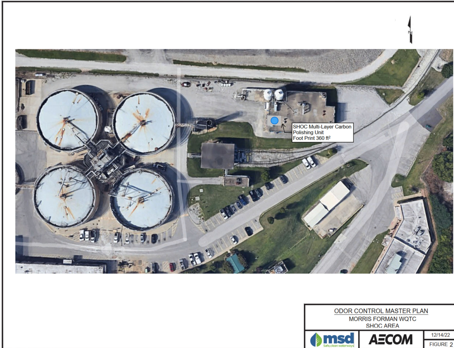
Figure 2 – SHOC Multi-Layer Carbon Polishing Area
